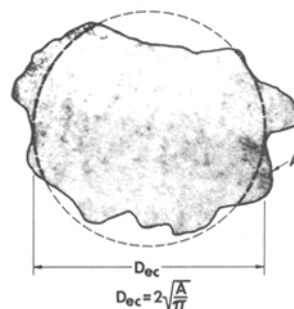
FIG. 3. The "Effective Circular Diameter" of a dust particle.
